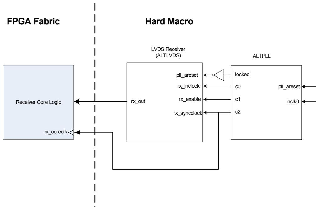
The two input ports, `rx_inclock` and `rx_enable`, to the LVDS receiver instance are available through the ALTLVDS MegaWizard Plug-In Manager. The ports `pll_areset` and `rx_syncclock` are not available through the ALTLVDS MegaWizard Plug-In Manager and must be manually included by modifying the `.v` or `.vhdl` wrapper file generated by the ALTLVDS MegaWizard Plug-In Manager.
