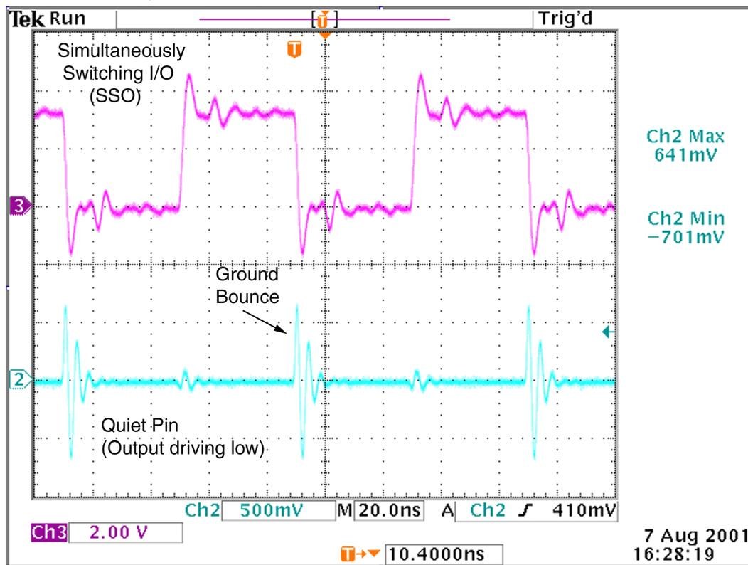
It is important to understand the mechanism for measuring the device ground, which is to monitor an I/O driving out low, commonly referred to as a quiet pin. Since ground pins are connected directly to the board ground, monitoring a ground pin will represent the board ground, not the internal device ground.
