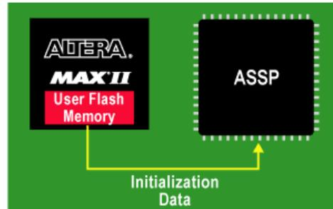
The UFM also can be used in board design where system designers are increasingly using serial EEPROMs instead of dual in-line package (DIP) switches and jumpers to configure their boards. This configuration data can control system parameters such as memory configuration, IP or port address, or peripheral address specification (e.g., USB).
