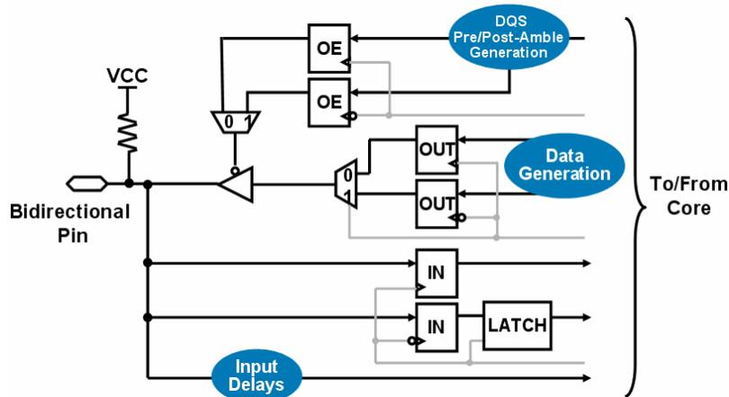
The advantage of having these registers in the IOE allows for minimum clock and data skew, which minimizes the degradation of the sampling window – this effectively allows Stratix II's DDR2 implementation to achieve high data rates with high reliability.
