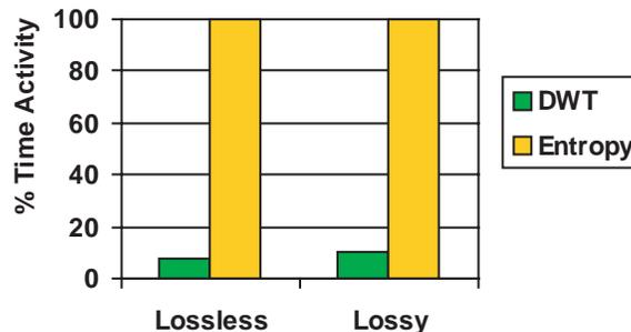
To compensate for this slow entropy encoding and to better balance the activity of the various blocks of the JPEG2000 encoding, several entropy encoders must be placed in parallel to independently process the code blocks generated by a single wavelet engine.
