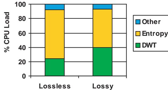
To increase the JPEG2000 performance, Barco Silex has developed an architecture where the computationally intensive wavelet, quantization, and entropy encoding tasks are off-loaded to an Altera® FPGA coprocessor, as illustrated in Figure 3.
