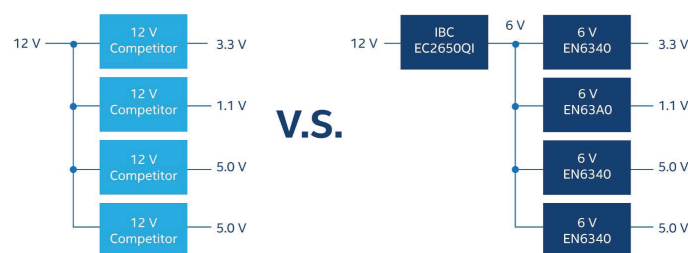
Figure 2. 1-Stage vs. 2-Stage Block Diagram Configuration
