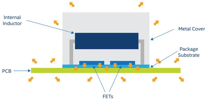
**Figure 1.** Thermal pathways removing heat from the Intel Enpirion PowerSoC package
