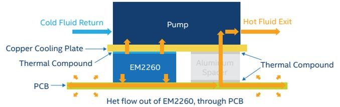
Figure 4. Thermal Conduction Pathways of the PowerSoC Package
