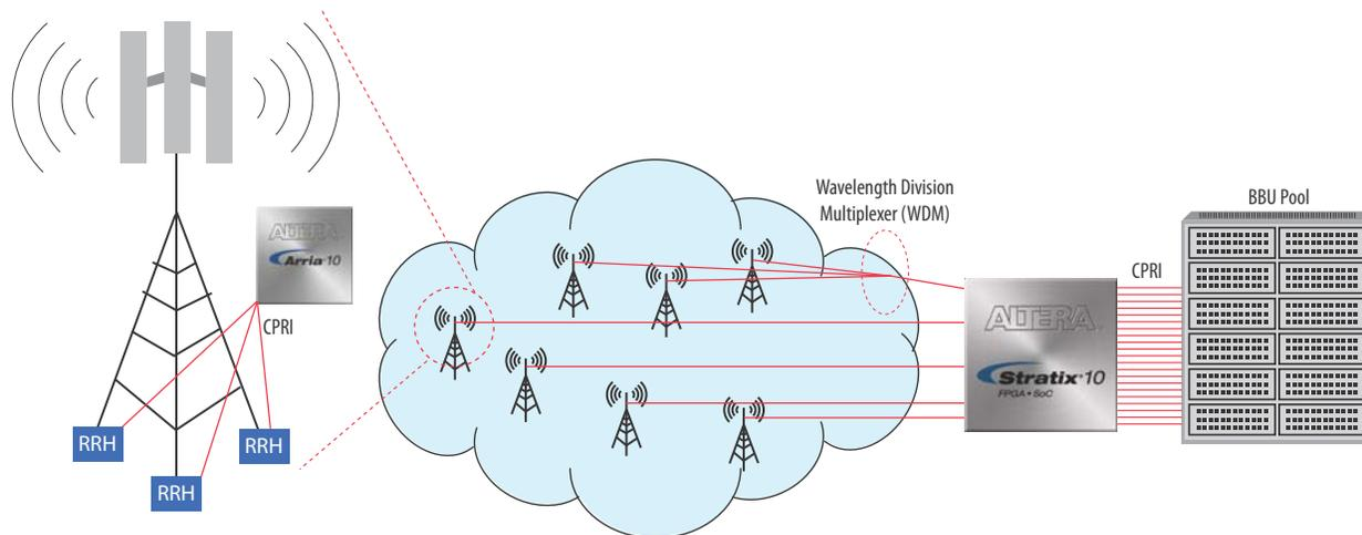
Altera, now part of Intel, offers FPGA technology and IP to implement integrated and re-programmable front-haul solutions. Altera conducted tests to compare two alternative CPRI over OTN solutions.
