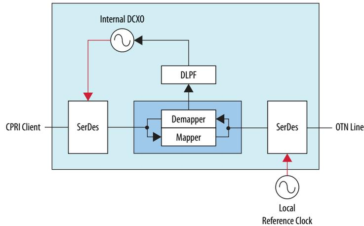
This timing information is low-pass filtered and then used to control the internal Arria 10 device DCXO. It provides the transmit reference clock for the CPRI client SerDes, effectively controlling the CPRI signal rate.
