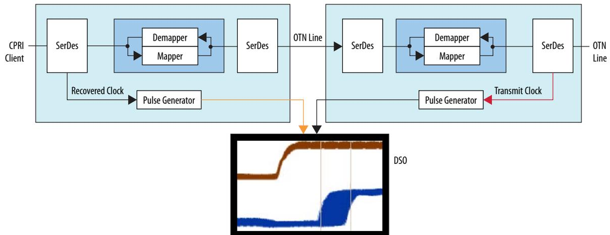
A DSO monitored the maximum variation in the delay between input and output over a given time period (e.g., 12 hours).
