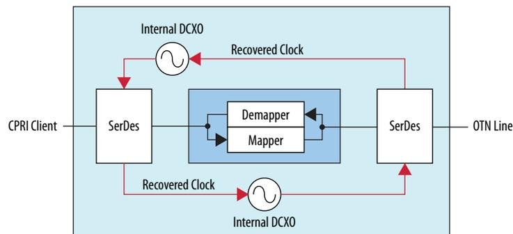
In this case, the transmit reference clocks for both CPRI and OTN signals were derived using the internal DCXO of the Arria 10 device.
