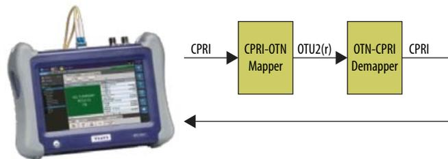
To initiate a complete restart of the system, the optical signals at both the CPRI and OTN sides are interrupted and then traffic is re-established. We then measured the latency. The test process repeated this sequence a number of times and we recorded the worst-case deviation from the average.
