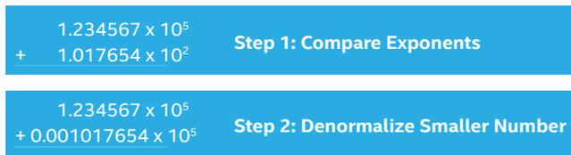
Figure 1. Preliminary Steps for Floating-Point Addition
