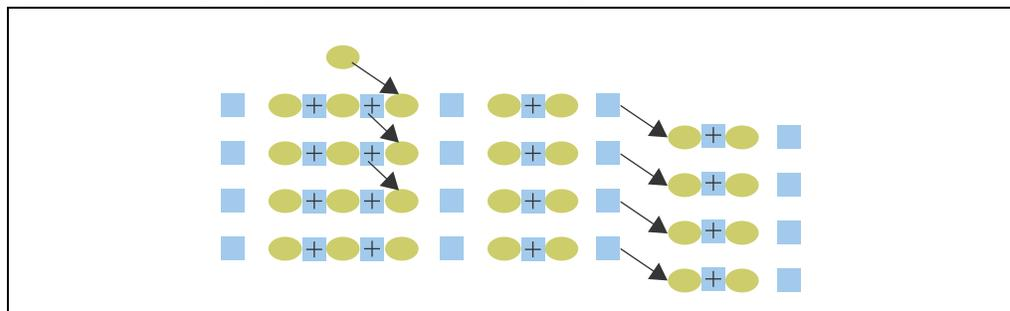
The final option involves deleting half of the width and retaining the original bandwidth. For highly parallel circuitry, this is the stopping point: twice the clock rate, same latency, and half the area (refer to [Figure 3](#)).
