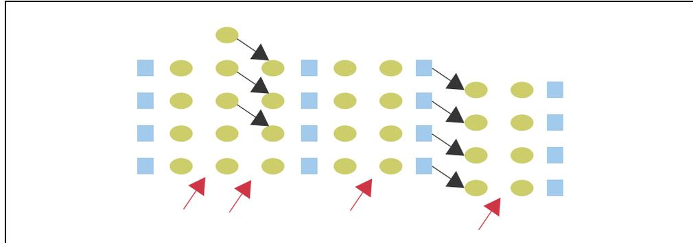
Matching unregistered LUTs with registers resulted in doubling the bandwidth of the circuit while retaining the same area. For example, a 100GbE could run at 200 Gbps. Applications engineers now had the option of either running two independent streams or running one stream on half the circuitry (refer to [Figure 2](#)).
