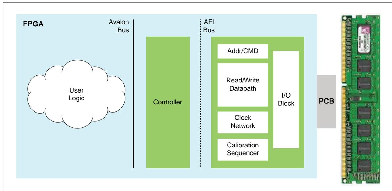
The memory interface is comprised of three parts:
