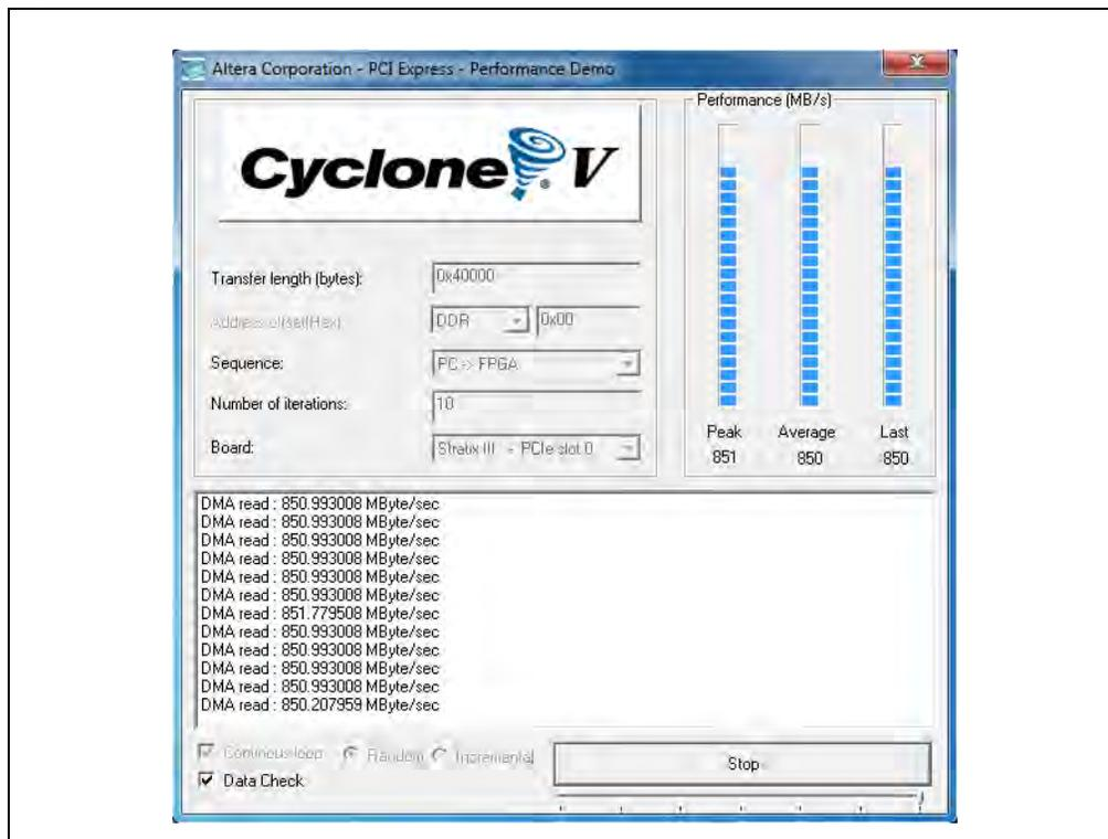
For writes, the actual bandwidth is 850 MBps. With a theoretical maximum of 920 MBps, where the system performance bottleneck is located, the PCIe controller is achieving a 92% utilization or efficiency level. Metrics slightly lower than the theoretical maximum are due to maximum theoretical calculations that did not take into account the additional protocol overhead for DLLP and PLPs. This overhead marginally reduces the real throughput depending on the traffic transmitted.
