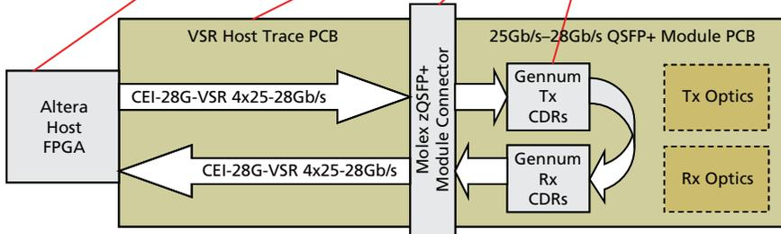
**Figure B: CEI-28G-VSR Interoperability Block Diagram and Setup**
