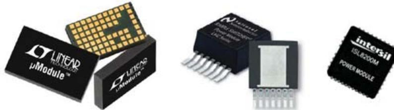
For example Linear Technology's  $\mu$ Module takes all components associated with the switching regulator circuit and encapsulates them on a substrate. The major blocks such as the DC/DC converter, MOSFETs, and Inductor reside on their own substrate and are interconnected. This technology further reduces the footprint and improves the optimization compared to the POLA and DOSA Modules. [Table 1](#) compares the footprint area of each package.
