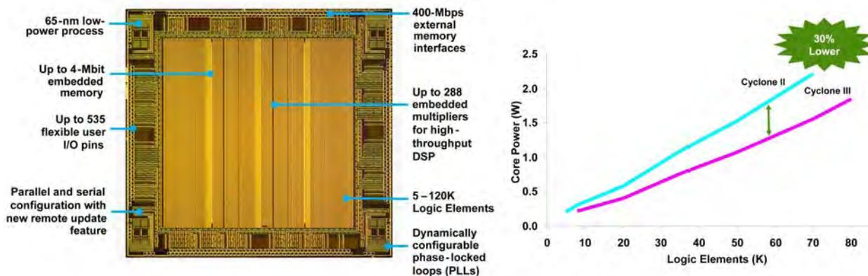
Embedded processing, once limited to ASIC implementations, is now available as an option in production FPGAs. As an example, Altera offers the Nios® II configurable processor core that supports up to 340 DMIPS with a single instantiation. The power saving benefit of a soft core processor over external microprocessors and microcontrollers further contributes to a more power-efficient data-recovery circuit.
