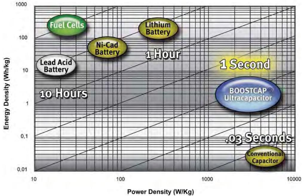
RAID adapter card specifications require short bursts of energy to provide sufficient power density for backing up data during power-down conditions. Capacitor technology supports these energy requirements through the physical law of
