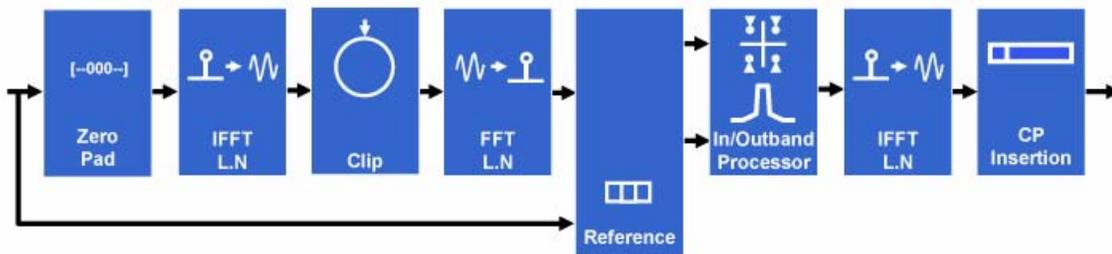
The system accepts data at the input as OFDM(A) symbols (of length  $N$  carriers) in the frequency domain. The first process is to upconvert the data by a factor  $L = 4$ , using perfect frequency domain interpolation (zero padding). The technique involves performing CFR at a higher sampling frequency as there is peak growth associated with upconversion. In addition, a higher sampling frequency spreads the non-linear distortions introduced by subsequent blocks across a larger bandwidth.
