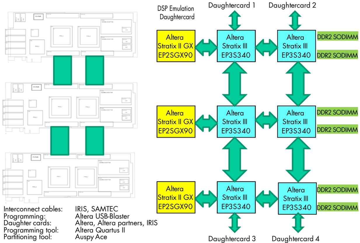
The most common use of FPGA-based prototyping platforms is for prototyping ASICs such as the one shown in Figure 3. For increasing the number of desired gates, boards can be daisy-chained or cross-connected using interconnect cables provided by IRIS Technologies as shown in Figure 8, Figure 9, and Figure 10, or in a system as shown in Figure 11.
