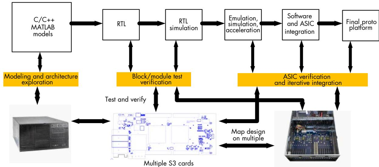
Figure 7 shows a more generic flow for an ASIC that includes system prototyping, simulation, and emulation.
