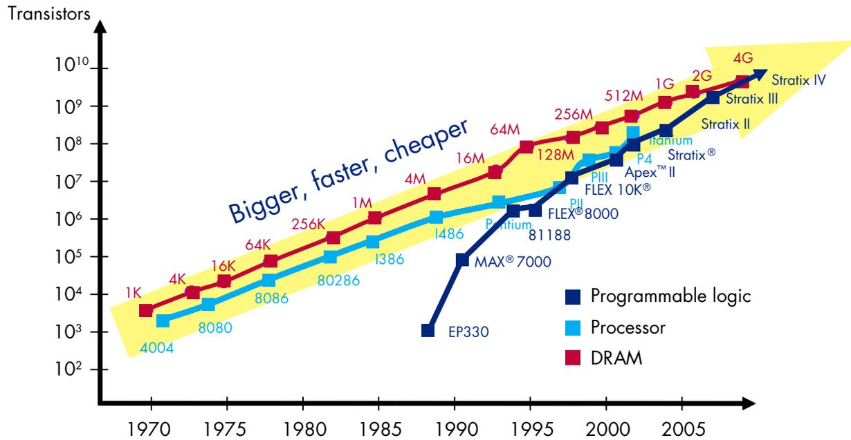
With these more complex devices come significant opportunities to consolidate complex algorithms, reduce component count, and create systems that are more flexible with FPGA designs. This flexibility comes at a potential cost in design effort and verification.
