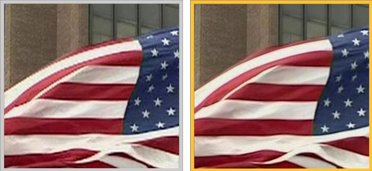
Measuring and predicting spatial motion can only go so far. One problem that cannot be solved in this manner is when two occluding blocks are moving in different directions. In this case, calculating the average motion creates an artifact. Alternate schemes to blur the results are not ideal and take additional processing power to detect and implement.
