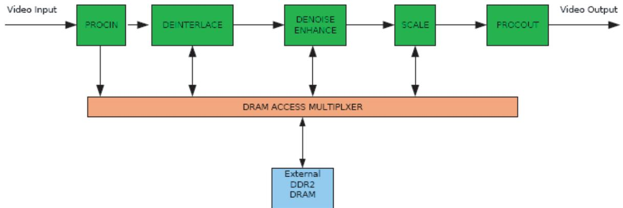
For the scaling stage, input pixels arrive in raster order, and without adequate internal memory, the pixels must be reordered through external memory and reread as partial lines before presentation to the vertical scaler. The pixels must also be reordered a second time to restore raster order before being sent to the horizontal scaler (see [Figure 6](#)).
