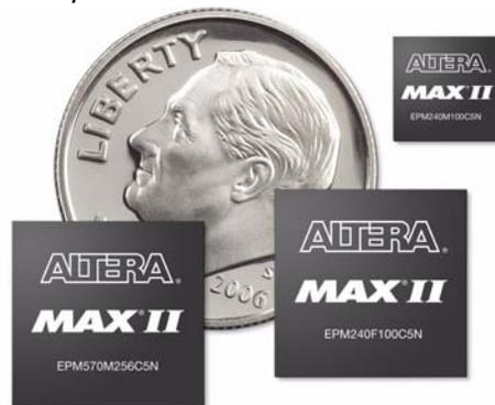
These small form-factor packages offer the compact size of a 0.5-mm BGA with the easy breakout of a partially populated array. The 68-pin, 100-pin, and 256-pin packages are designed so that all pins and power connections can be broken out with only two layers of the PCB using Micro Via PCM layout rules. (The 144-pin package requires four layers.)
