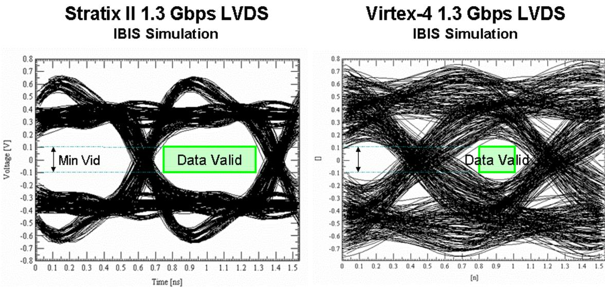
In Figure 4, Stratix II and Virtex-4 LVDS I/O signals are compared at 1.0Gbps data rates. The Stratix II eye is significantly cleaner, with 6.5 times less edge noise, a 3 times faster edge rate, and a 2.0 times wider data valid window.
