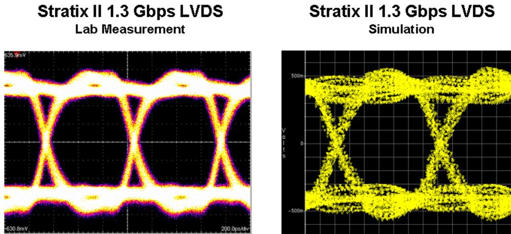
In Figure 3, Stratix II and Virtex-4 LVDS I/O signals are compared at 1.3 Gbps data rates. The Stratix II eye is significantly cleaner, with three times less edge noise, a three times faster edge rate, and a 2.3 times wider data valid window.
