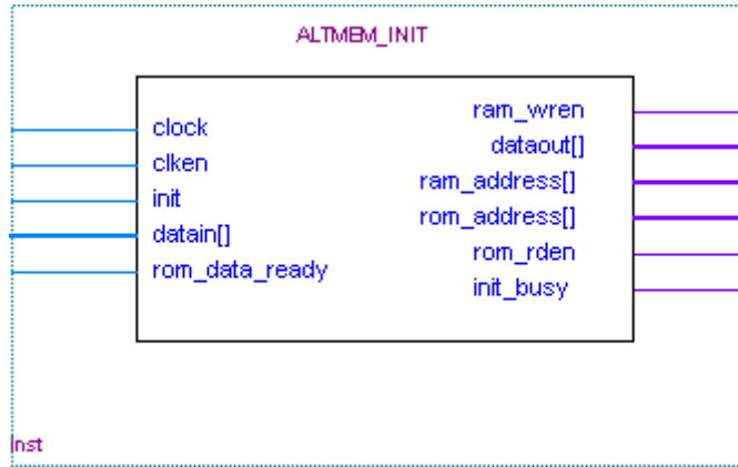
Figure 1–1. Input and Output Ports of ALTMEM_INIT Megafunction
