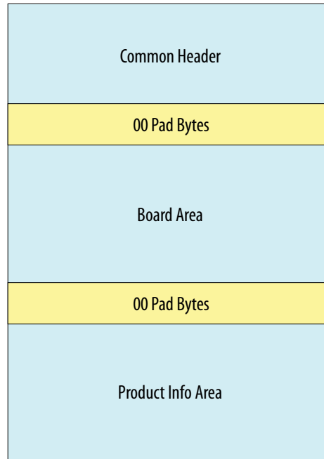
Figure 3. FRUID EEPROM Memory Layout Block Diagram
