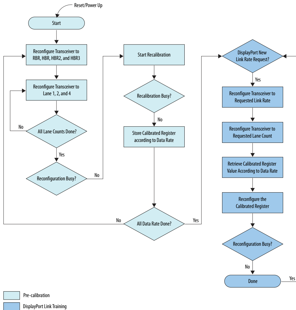
Figure 12. Transceiver Reconfiguration Flowchart
