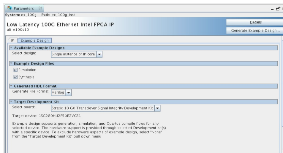
Figure 6. Example Design Tab in the Low Latency 100G Ethernet Intel Stratix 10 FPGA Parameter Editor
