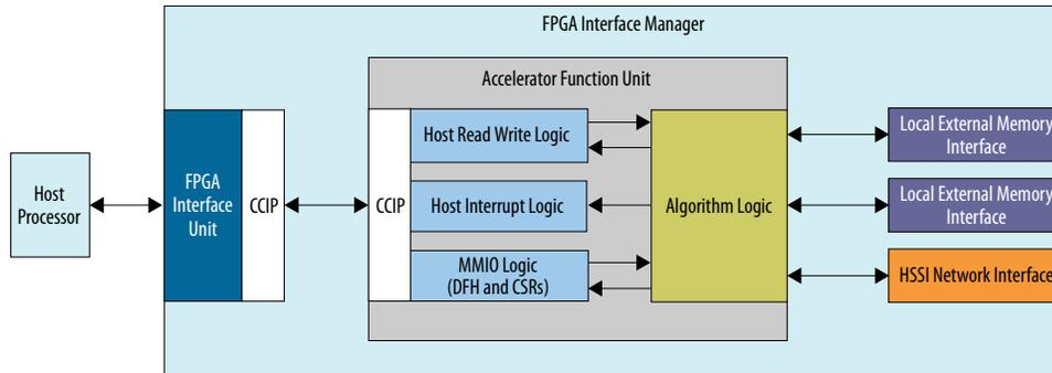
A typical AFU design includes the following components:
