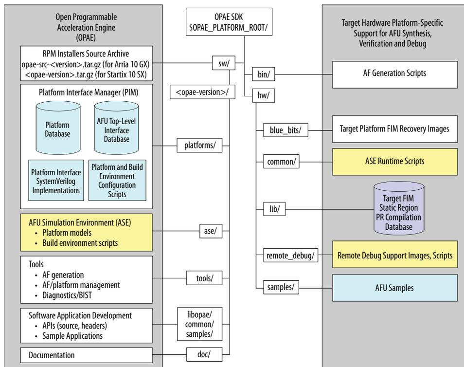
OPAE's Platform Interface Manager (PIM) defines a non-hardware specific OPAE Platform that provides generic classes of device interfaces. The OPAE platform is an abstraction of a hardware platform for which AFUs are designed. This level of abstraction enables generating AFs from AFUs designed for the generic OPAE Platform for any OPAE-compliant hardware platform that offers the device interfaces required
