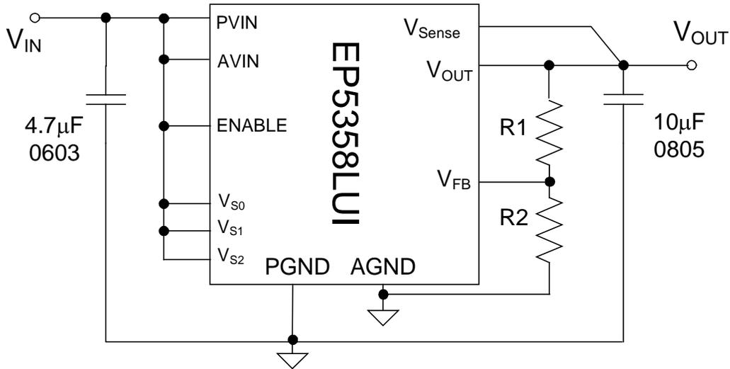
Figure 3. External divider schematic for the EP5358LUI.
