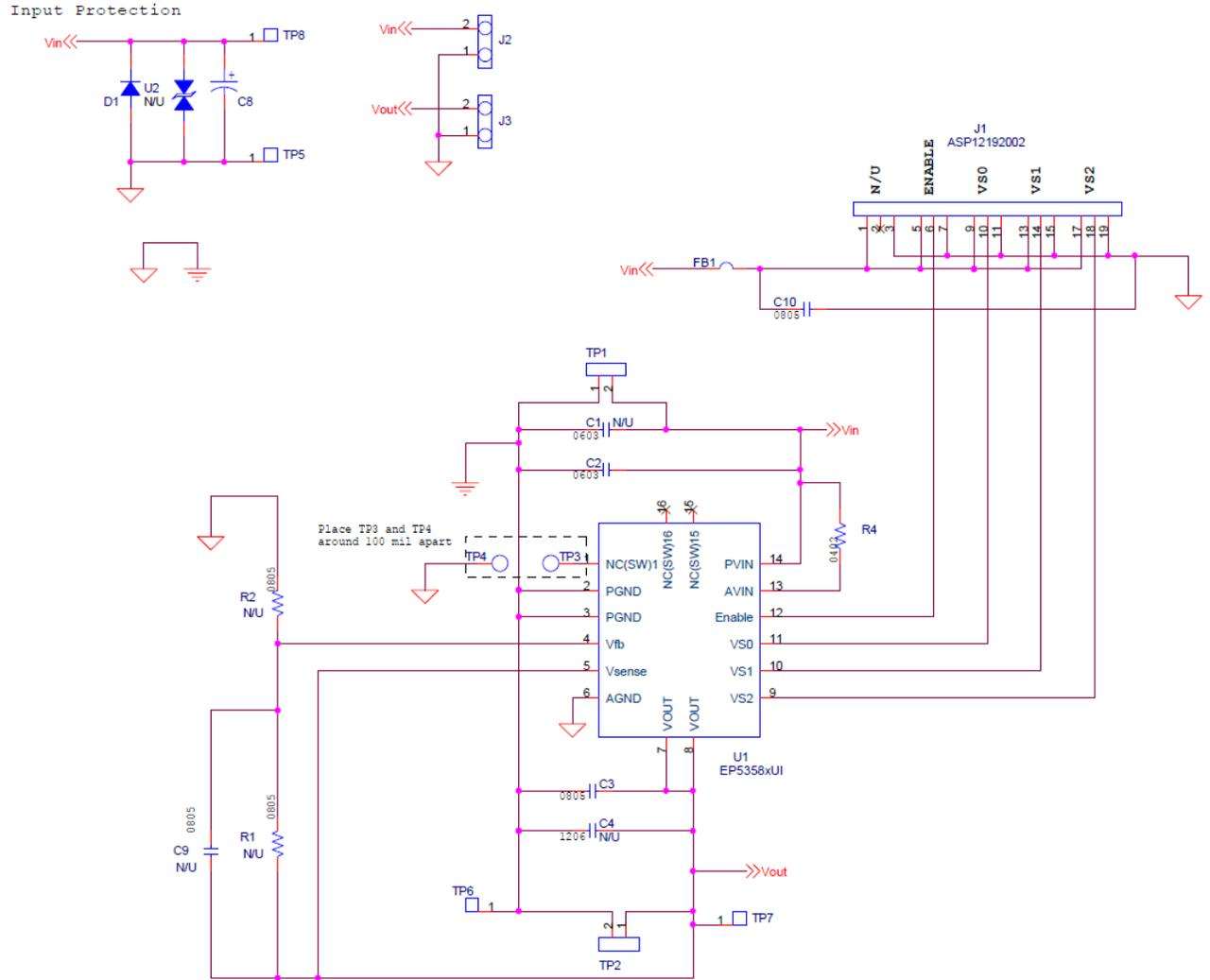
**Figure 5. 2.5mmx2.25mm Module Evaluation Board Schematic**
