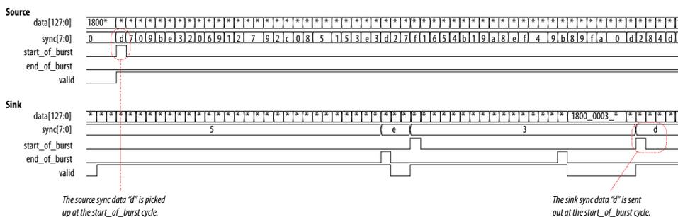
**Figure 12. Sink Waveform for Continuous Mode**
