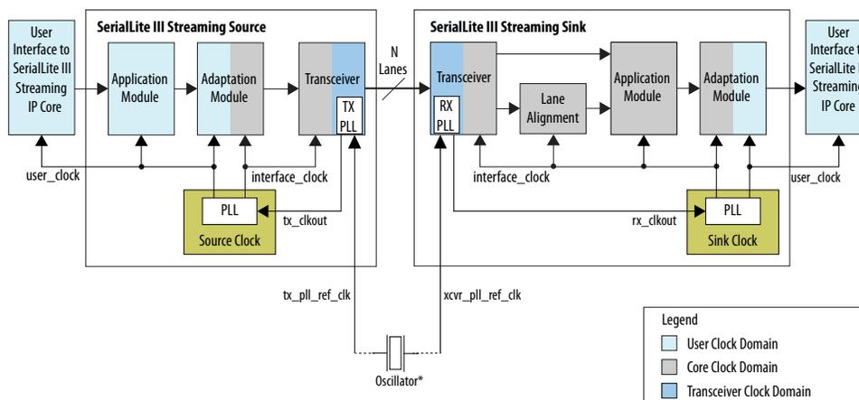
\*Intel recommends connecting tx\_pll\_ref\_clk and xcvr\_pll\_ref\_clk to the same oscillator to eliminate PPM differences between source and sink cores.
