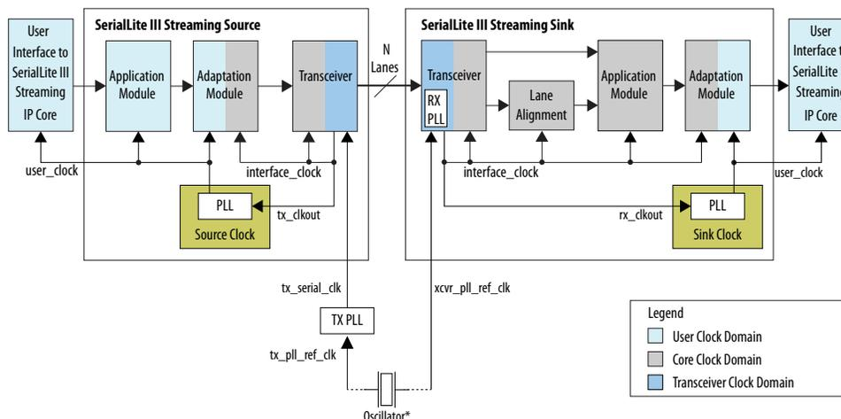
\*Intel recommends connecting tx\_pll\_ref\_clk and xcvr\_pll\_ref\_clk to the same oscillator to eliminate PPM differences between source and sink cores.
