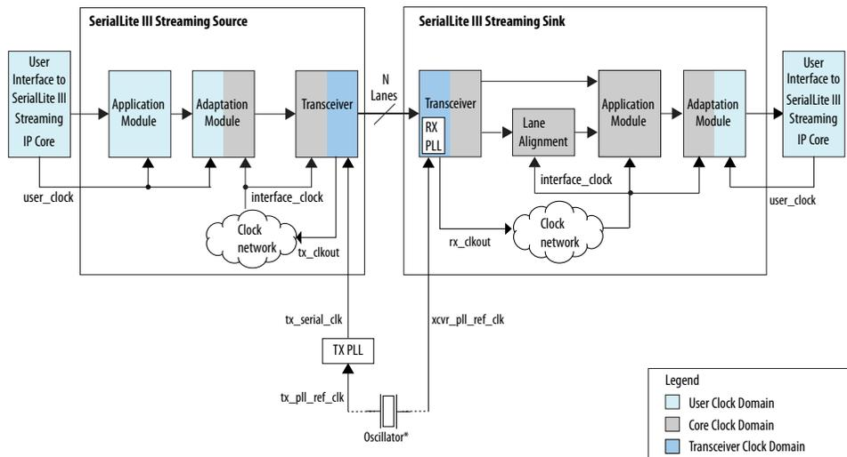
\*Intel recommends connecting tx\_pll\_ref\_clk and xcvr\_pll\_ref\_clk to the same oscillator to eliminate PPM differences between source and sink cores.
