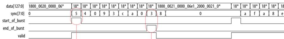
*The source sync data are picked up at the start\_of\_burst and end\_of\_burst cycle.*
