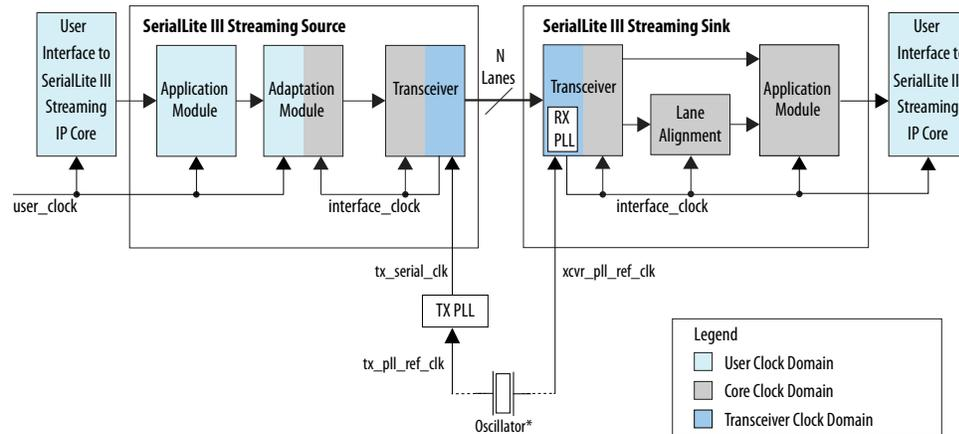
\*Intel recommends connecting tx\_pll\_ref\_clk and xcvr\_pll\_ref\_clk to the same oscillator to eliminate PPM differences between source and sink cores.
