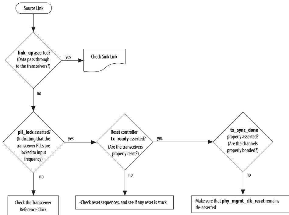
Table 38. Source Link Debugging Signals (Intel Arria 10, Intel Stratix 10, Arria V GZ, and Stratix V devices)
