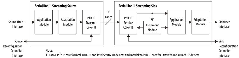
Figure 6. SerialLite III Streaming IP Core Duplex Core
