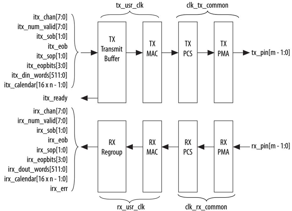
**Figure 10. Interlaken IP Core Block Diagram for E-Tile PAM4 Mode Device Variations**
