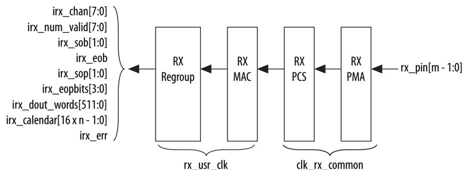
**Figure 14. Interlaken IP Core Receive Path Blocks for E-Tile PAM4 Mode Device Variations**
