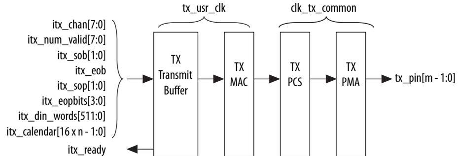
**Figure 12. Interlaken IP Core Transmit Path Blocks for E-Tile PAM4 Mode Device Variations**
