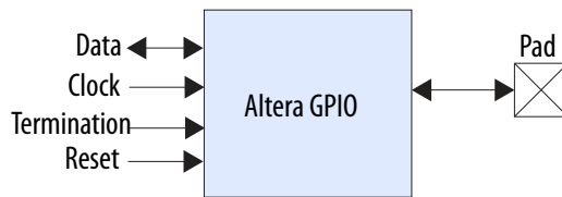
Figure 6. Altera GPIO IP Core Interfaces
