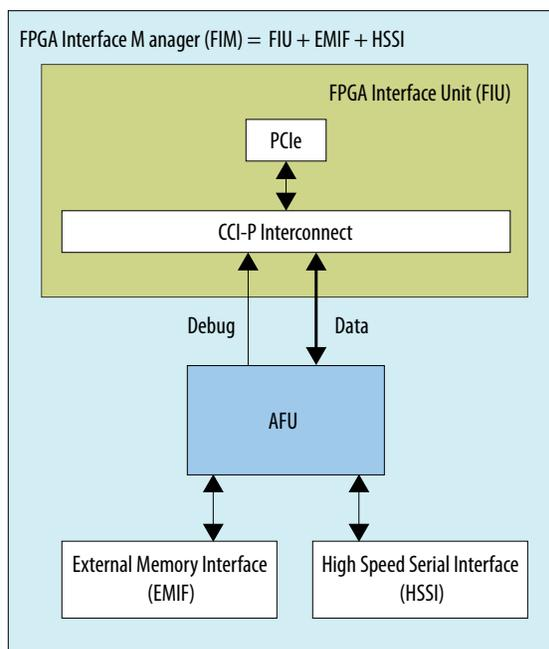
The AFU connects to the Intel Xeon processor through the CCI-P interface and then the PCIe link. The Intel PAC with Intel Arria 10 GX FPGA platform uses a simplified version of the CCI-P interface. For more information about the CCI-P interface, refer to the *Intel Acceleration Stack for Intel Xeon CPU with FPGAs Core Cache Interface (CCI-P) Reference Manual*.
