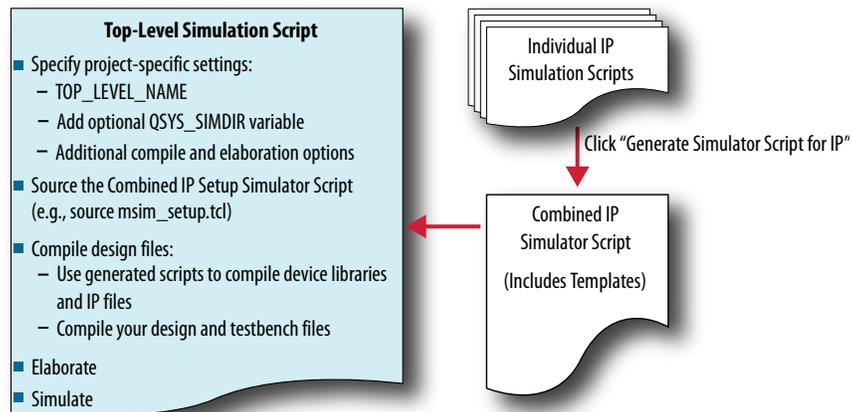
1. Click **Project > Upgrade IP Components > Generate Simulator Script for IP** (or run the `ip-setup-simulation` utility) to generate or regenerate a combined simulator setup script for all IP for each simulator.
