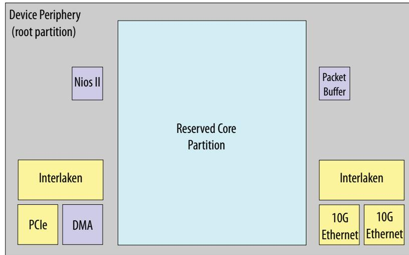
You can reuse the root partition with multiple other boards. The root partition Developer creates a design that meets expected design requirements with all the required resources, while also reserving a region (the reserved core) for Consumer development. The Developer then exports the root partition as a .qdb file and passes the .qdb to the Consumers of the partition.
