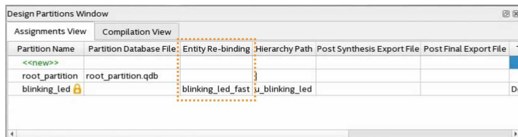
In a root partition reuse example, the Developer's project includes the shell with entity name blinking\_led, and the u\_blinking\_led instance. The Developer exports the root\_partition.qdb that includes the root partition, and a reserved core region defined by a Logic Lock placement constraint. The reserved region is associated with the u\_blinking\_led instance.
