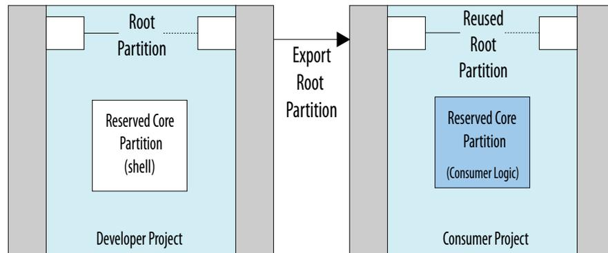
In root partition reuse, each project must target the same Intel FPGA part number, must have the same interfaces, and use the same version of the Intel Quartus Prime Pro Edition software. The following example shows reuse of an optimized root partition that contains various periphery interfaces. Only the reserved core partition that contains custom logic changes between Consumer projects.
