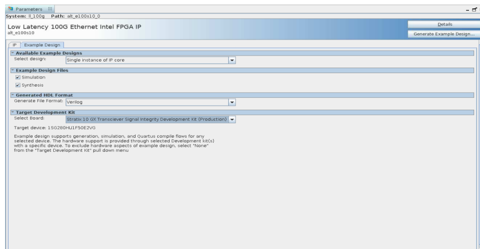
Figure 6. Example Design Tab in the Low Latency 100G Ethernet Intel Stratix 10 FPGA Parameter Editor
