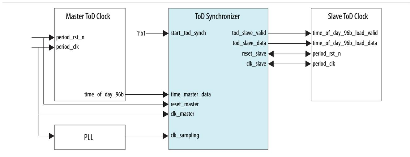
The ToD synchronizer uses a dual-clock FIFO buffer to receive the time of day from the master ToD clock and transmits it to the slave ToD clock. To ensure that the synchronization is accurate, the transfer latency must be taken into consideration. The sampling clock (`clk_sampling`) samples the fill level of the FIFO buffer and calculates the latency. Derive this clock signal from the same source as the master ToD clock or the slave ToD clock using a PLL.
