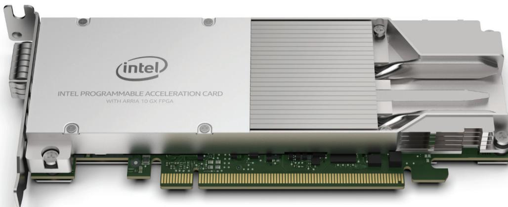
**Figure 3.** Intel Programmable Acceleration Card with the Intel Arria 10 GX FPGA
