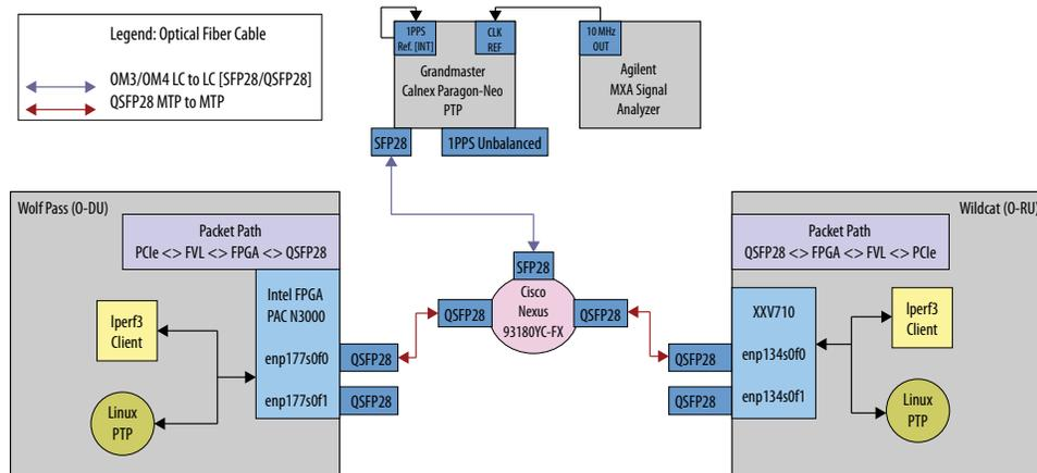
The PTP4I output on each of the DUT hosts provides data measurements of the PTP performance for each slave device in the setup (Intel FPGA PAC N3000 and XXV710). For `iperf3` traffic test, the following conditions and configurations apply to all graphs and performance analysis:
