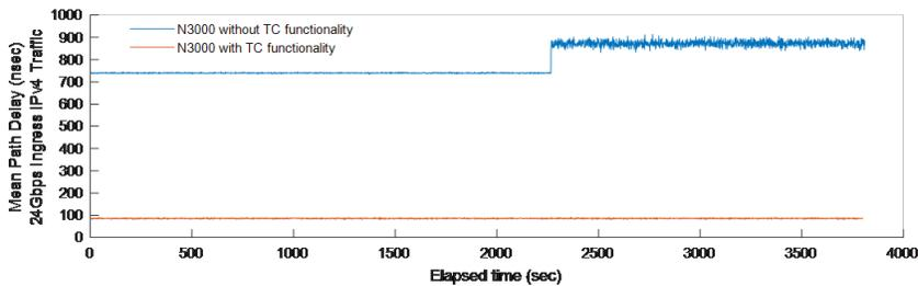
These figures show the PTP4I slave’s servo algorithm, due to the residence time correction of the TC, we see small differences in the average path delay calculations. Therefore, the impact of the delay fluctuations on the master offset approximation is reduced.
