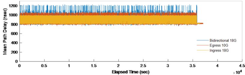
Regarding the Intel FPGA PAC N3000 PTP performance, the worst-case master offset under any traffic condition is within 90 ns. While under the same bidirectional traffic conditions, the RMS of the Intel FPGA PAC N3000 master offset is 5.6x better than the one of XXV710 card.
