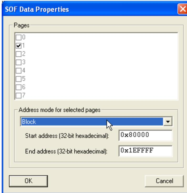
A sample memory map output file for the preceding example is shown below. Note that the allocated memory for page 1 is between 0x00080000 and 0x001EFFFF, while the actual region used by the current application configuration bitstream is between 0x001AB36C and 0x001EFFF7. The configuration data is top justified within the allocated SOF data region.
