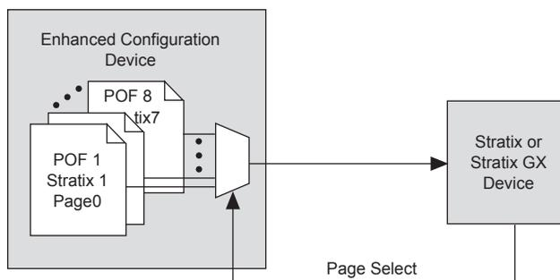
Upon power-up in remote configuration mode, the factory configuration (see description below) selects the user-specified page address through the Stratix or Stratix GX PGM[2..0] output pins. These pins drive the PGM[2..0] input pins of the enhanced configuration device and select the requested page in the memory.
