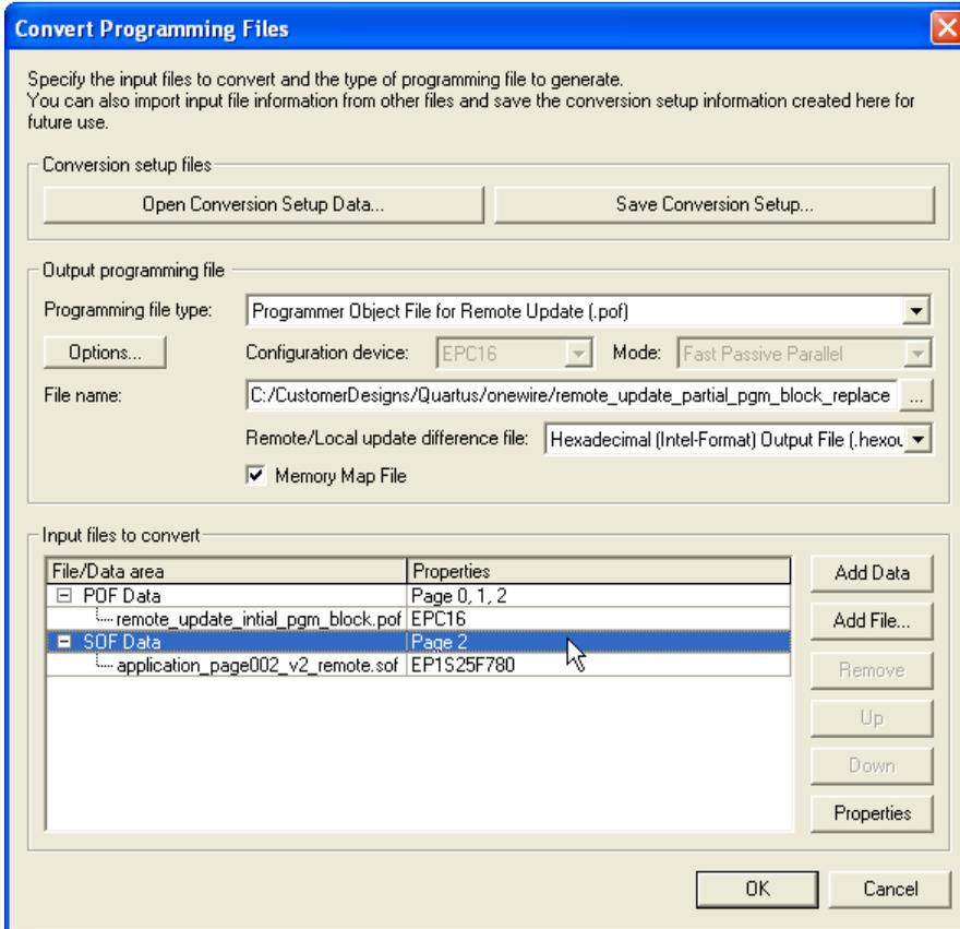
Figure 12–24. Specifying Block Addresses for Application Configuration
