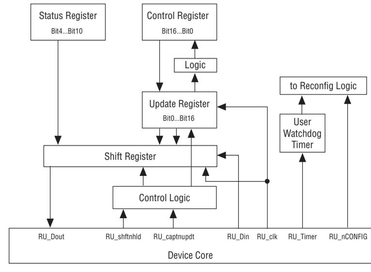
Table 12–3 describes the user configuration signals that are driven to/from the device logic array. The remote configuration logic has one input signal to the device logic array and six output signals from the device logic array.
