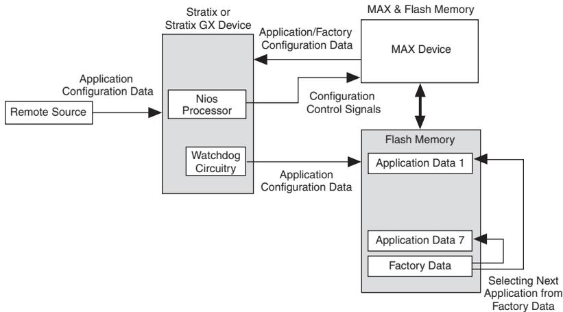
You can use both remote and local configuration modes in this scheme. You should specify a default page for factory configuration and make sure it is not altered or removed at any time. In remote system configuration mode, PS, FPP, and PPA modes are supported when configuring with MAX and flash devices.
