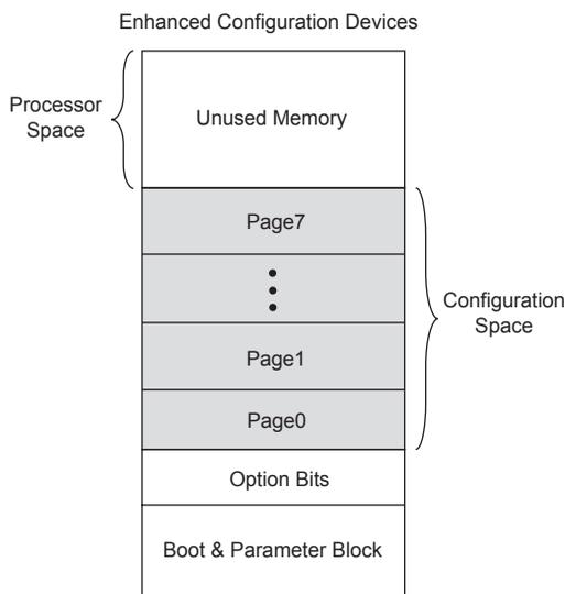
When the Stratix or Stratix GX device powers-up in remote configuration mode, the device loads configuration data located at page address 000. You should always load the factory default configuration data at this location and make sure this information is not altered.
