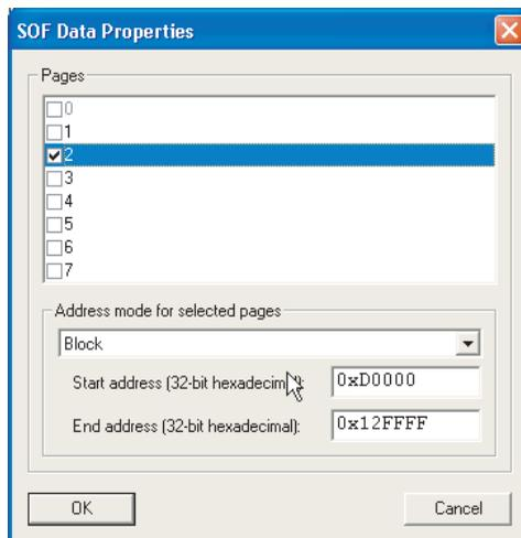
For adding a new application configuration, follow the steps listed above with one modification. In Step 5, select **SOF Data** and click on **Properties**. In the **SOF Data Properties** dialog box, select a new page (for example, page 3) and specify the addressing mode information. Continue with steps 7 through 10. When a new page is added, the memory map output file lists the start/end addresses for this page. A sample is shown below:
