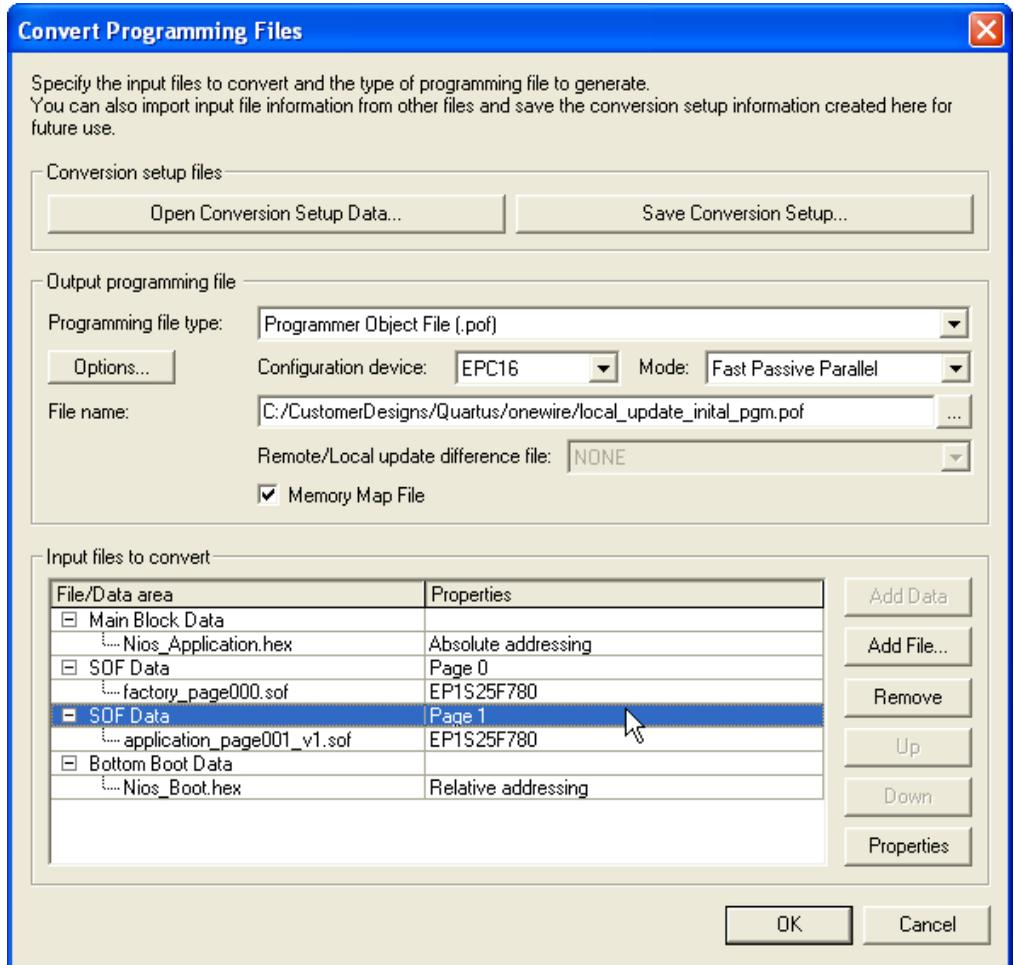
Figure 12–15. Specifying Block Addresses for Application Configuration
