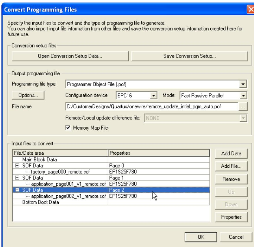
A sample memory map output file for the preceding setup is shown below. Notice all configuration pages are packed such that two pages can share a flash data sector. This disallows partial programming of application configurations in auto addressing mode.
