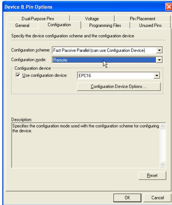
Additionally, the remote configuration mode requires you to either instantiate the `altremote_update` megafunction or the WYSIWYG (what-you-see-is-what-you-get) atom into your design. Without this atom or megafunction, you are not able to access the dedicated remote configuration circuitry or registers within the Stratix or Stratix GX device. See [Figure 12–10](#) for a symbol of the `altremote_update` megafunction.
