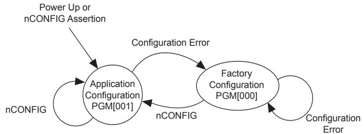
In local configuration mode, one application configuration is available to the device. For remote or local configuration mode selection, see [Table 12–1](#).
