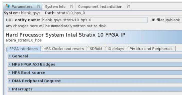
Figure 2. HPS Component Parameter Editor FPGA Interfaces Tab
