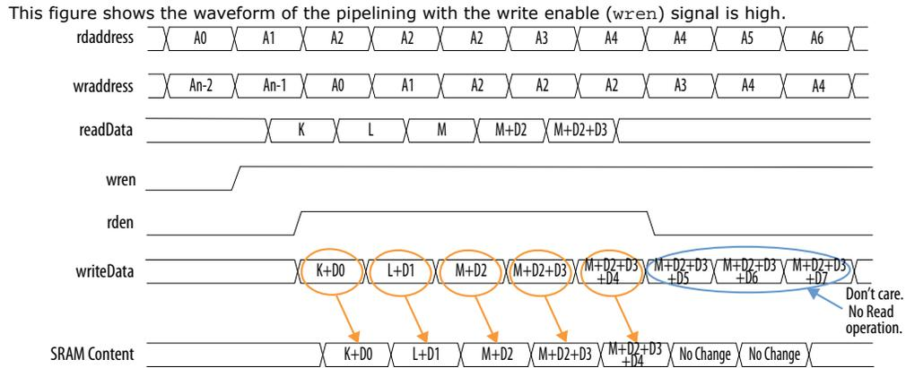
With the coherent read feature enabled and forwarding logic implemented, the output of M20K blocks can be either unregistered or registered. To match the latency of the coherency circuitry within the hardware boundary of the M20K blocks, you may need to manually add the additional pipeline registers on the *wren* and *wraddress* paths, which is described in the following table:
