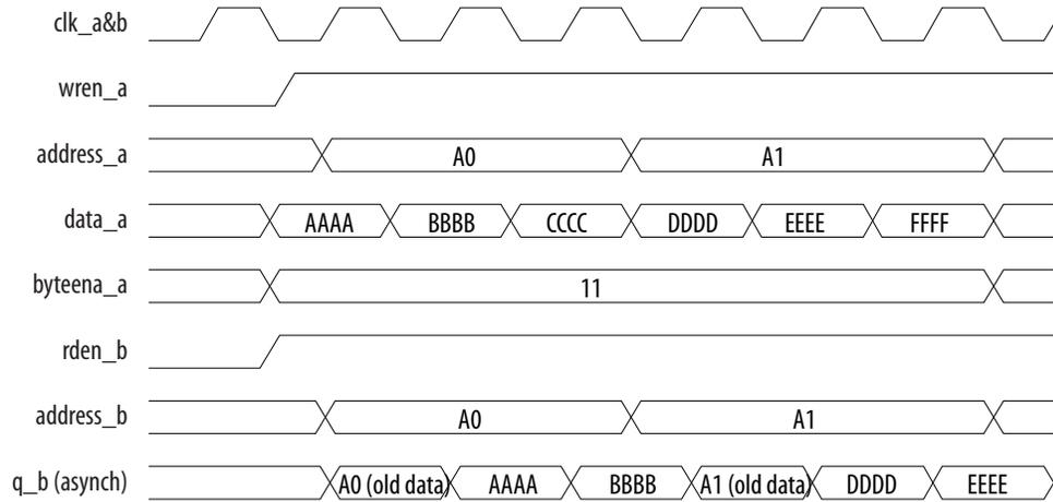
**Figure 23. Mixed-Port Read-During-Write: *Don't Care Mode***
