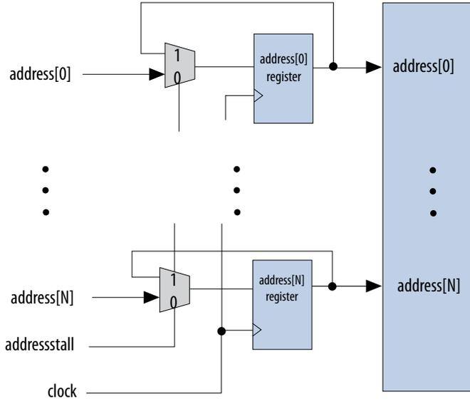
**Figure 3. Address Clock Enable During Read Cycle**
