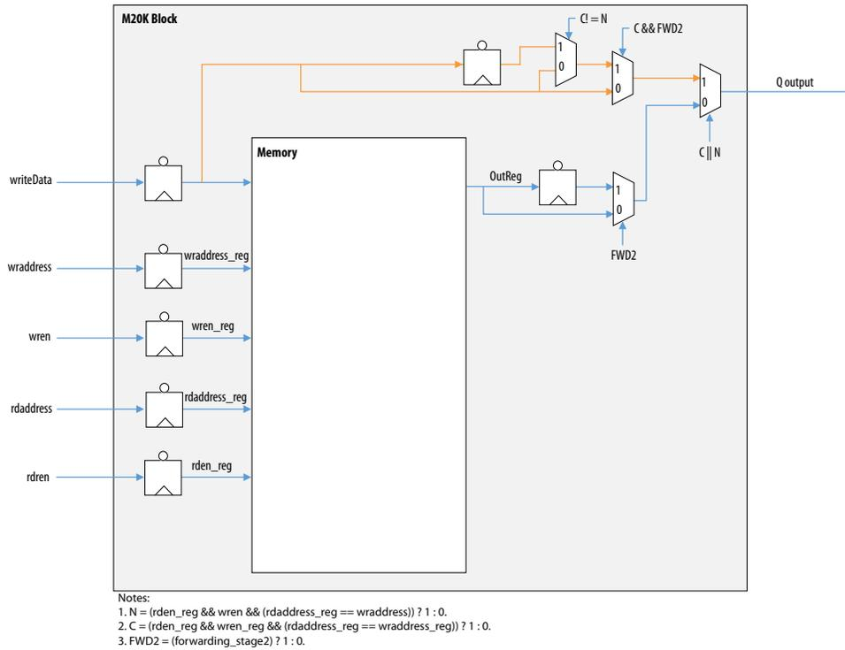
Figure 9. Coherent Read Memory Behavior for Unregistered Output
