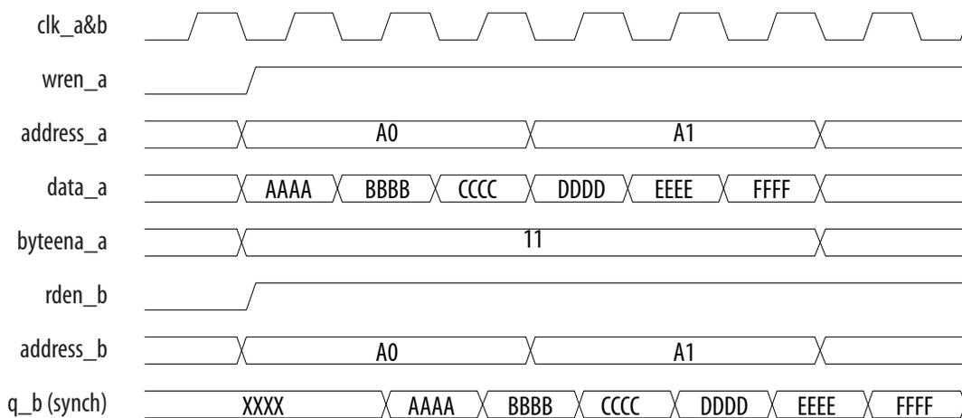
**Figure 22. Mixed-Port Read-During-Write: *Old Data Mode***
