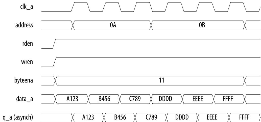
**Figure 20. Same-Port Read-During-Write: Don't Care Mode**
