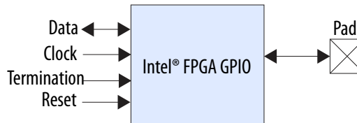
Figure 37. Intel FPGA GPIO Interface Signals
