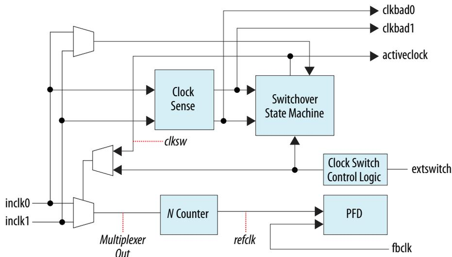
When the current reference clock is not present, the clock sense block automatically switches to the backup clock for I/O PLL reference. You can select a clock source as the backup clock by connecting it to the `inclk1` port of the I/O PLL in your design.
