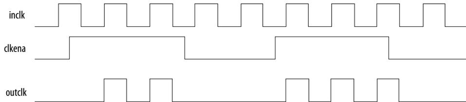
The clock signal going into the SCLK network in a sector can only reach the core logic in that sector. When you instantiate a SCLK gate in your design, the Intel Quartus Prime software automatically duplicates the SCLK gate to create a clock gate in every sector to which the clock signal is routed.
