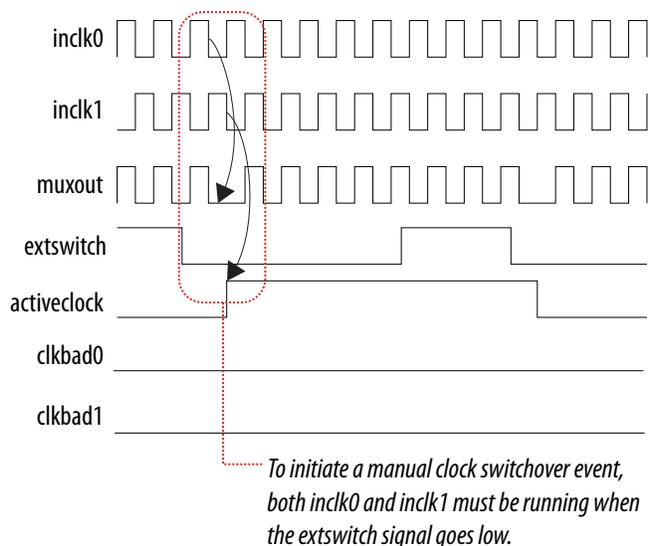
In automatic override with manual switchover mode, the `activeclock` signal inverts after the `extswitch` signal transitions from logic high to logic low. Since both clocks are still functional during the manual switch, neither `clkbad` signal goes high. Because the switchover circuit is negative-edge sensitive, the rising edge of the `extswitch` signal does not cause the circuit to switch back from `inclk1` to `inclk0`. When the `extswitch` signal goes low again, the process repeats.
