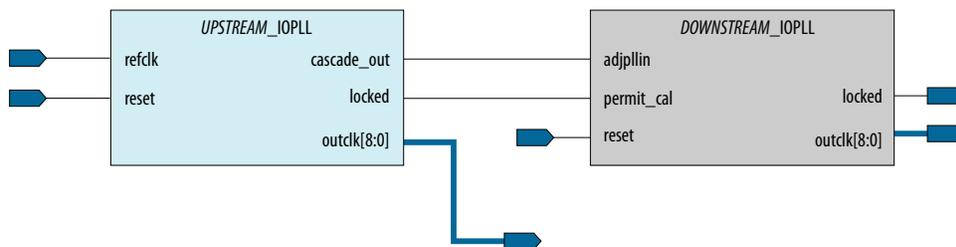
**Figure 17. I/O-PLL-to-I/O-PLL Cascading Via Core Clock Fabric**
