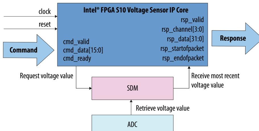
The SDM samples the voltage at regular intervals. When the Intel FPGA S10 Voltage Sensor IP core sends voltage sampling request to the SDM, the SDM returns the most recently read voltage value. The IP core then returns the observed voltage value as an unsigned 32-bit fixed point binary number.
