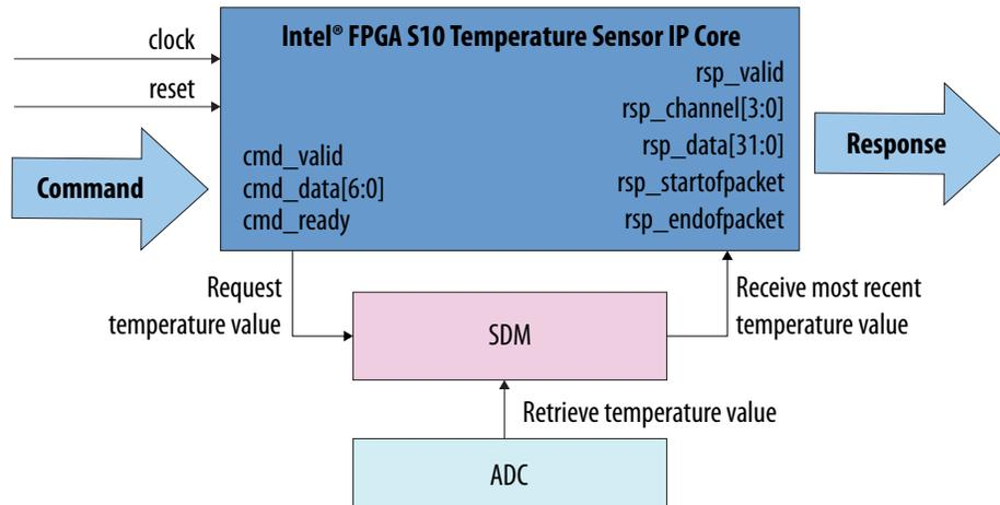
The SDM samples the temperature at a regular interval. When the Intel FPGA S10 Temperature Sensor IP core sends temperature sampling request to the SDM, the SDM returns the most recently read temperature value. The IP core then returns the observed temperature value in Celsius as a signed 32-bit fixed point binary number.
