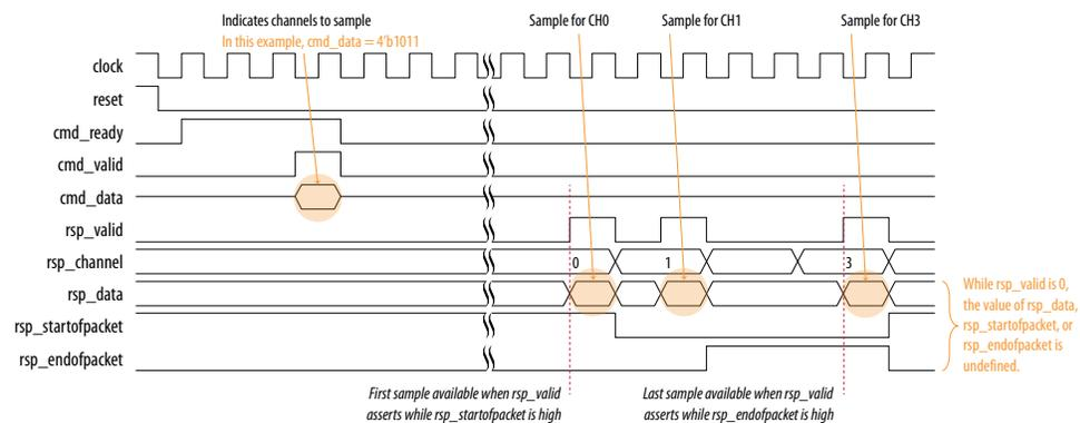
**Note:** Set only valid bits in the `cmd_data` word. Otherwise, the response from the temperature sensor is undefined.
