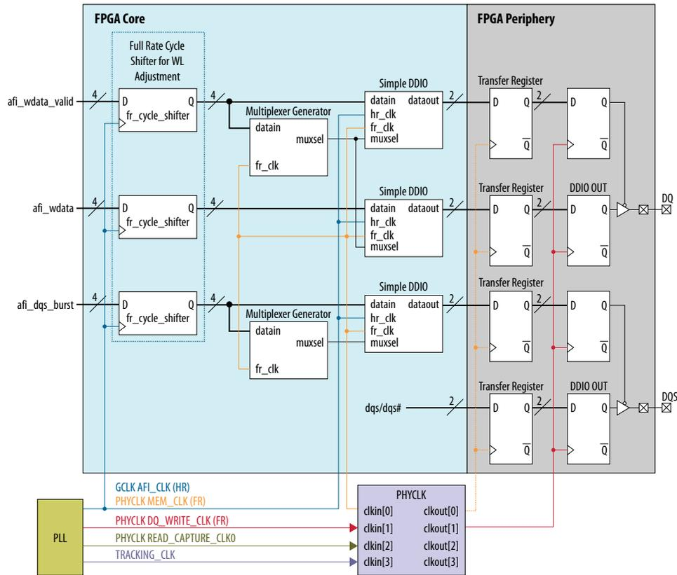
Figure 6. External Memory Interface Write Datapath Timing
