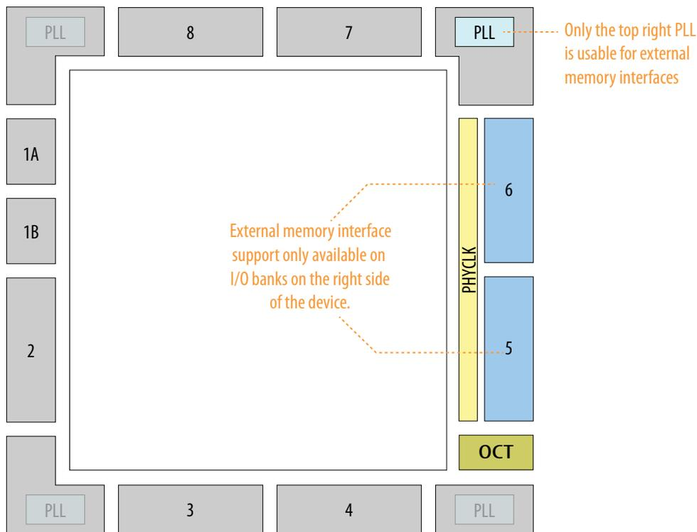
External memory interfaces support is available only for dual supply (DC, DF, and DA) variant on 10M16, 10M25, 10M40, and 10M50 devices.
