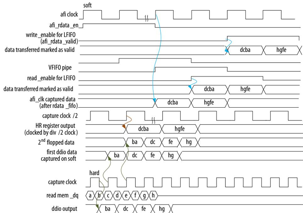
In Intel MAX 10 external memory interfaces, post-amble is not a concern because the read data strobe signal, DQS, is not used during read operation.
