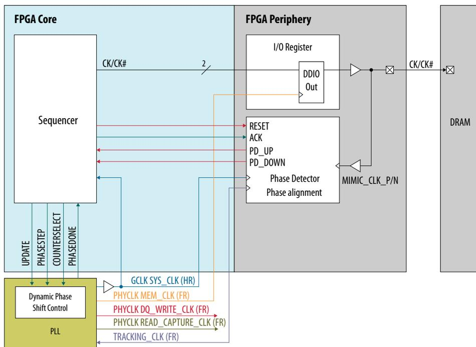
In the Intel MAX 10 external memory interface solution, the memory clocks are used to mimic the read and write paths. The memory clock pins loop back to the phase detector as a mimic clock. The phase detector provides any variation of the mimic clock to the sequencer. The sequencer adjusts the read capture clock to match the clock phase change.
