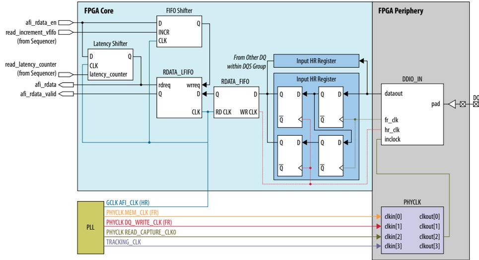
Figure 4. External Memory Interface Read Datapath Timing
