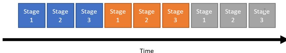
If each stage of this loop takes one clock cycle to execute, then this loop has a latency of nine cycles.
