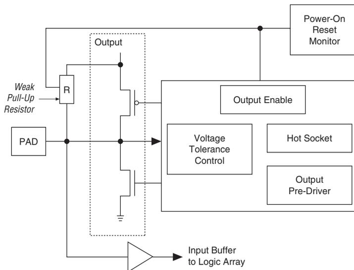
The POR circuit monitors  $V_{CCINT}$  voltage level and keeps I/O pins tri-stated until the device is in user mode. The weak pull-up resistor (R) from the I/O pin to  $V_{CCIO}$  keeps the I/O pins from floating. The voltage tolerance control circuit permits the I/O pins to be driven by 3.3 V before  $V_{CCIO}$  and/or  $V_{CCINT}$  are powered, and it prevents the I/O pins from driving out when the device is not in user mode.
