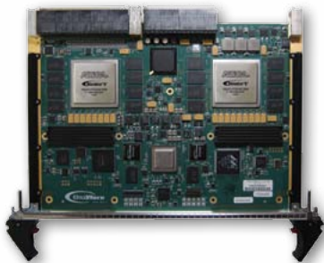
Figure 2: Bittware VPX board supporting the Altera EW ultra-wideband channelizer reference design
