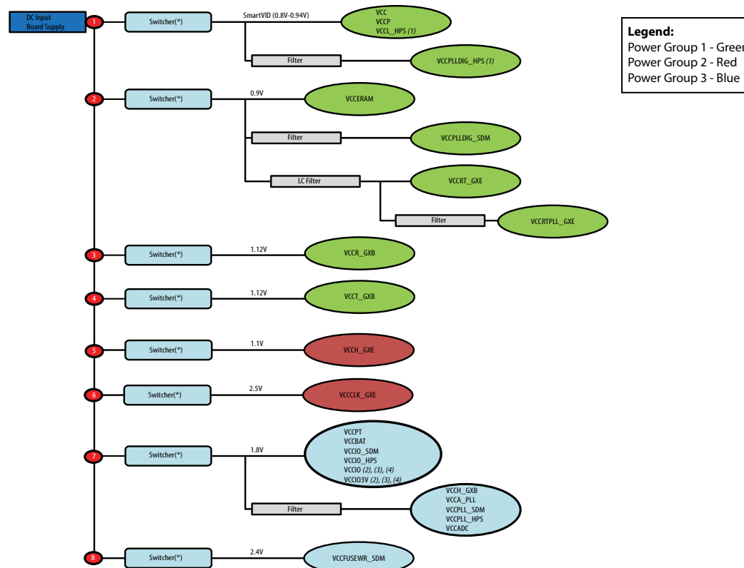
Figure 9. Example Power Supply Sharing Guidelines for Intel Stratix 10 TX (-1V, -2V, and -3V parts) with 10 Gbps < Transceiver Data Rate <= 57.8 Gbps—Preliminary
