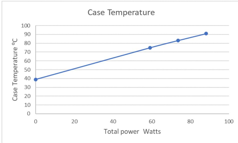
The above graph shows that the effective  $\Psi_{CA}$  is  $0.6^{\circ}\text{C}/\text{W}$  and the effective ambient temperature is  $40^{\circ}\text{C}$ .
