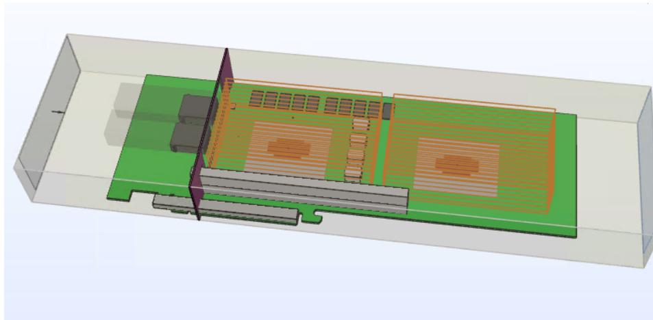
For purposes of this example, let's assume that the design targets a 35°C data center environment, and airflow over the card is 20 CFM. Using the methodology described above, we perform three sets of CFD analysis, for FPGA core die powers of 43.5 W, 58 W and 72.5 W.
