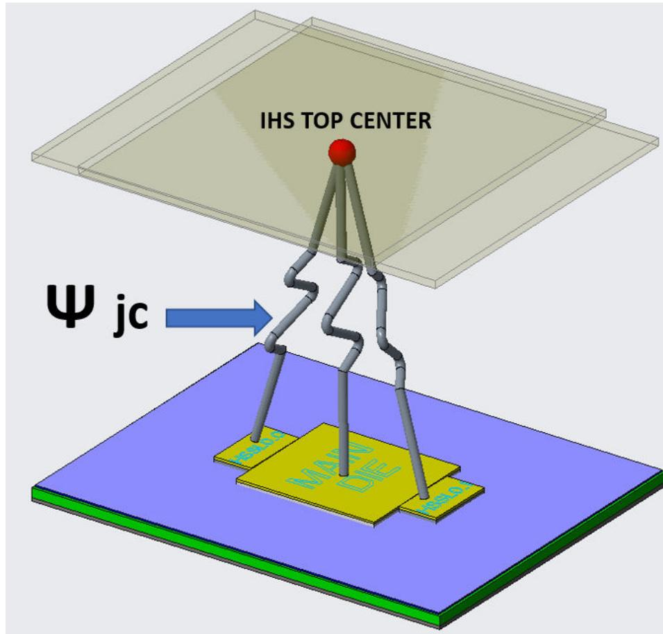
**Figure 3. Thermal Resistance**
