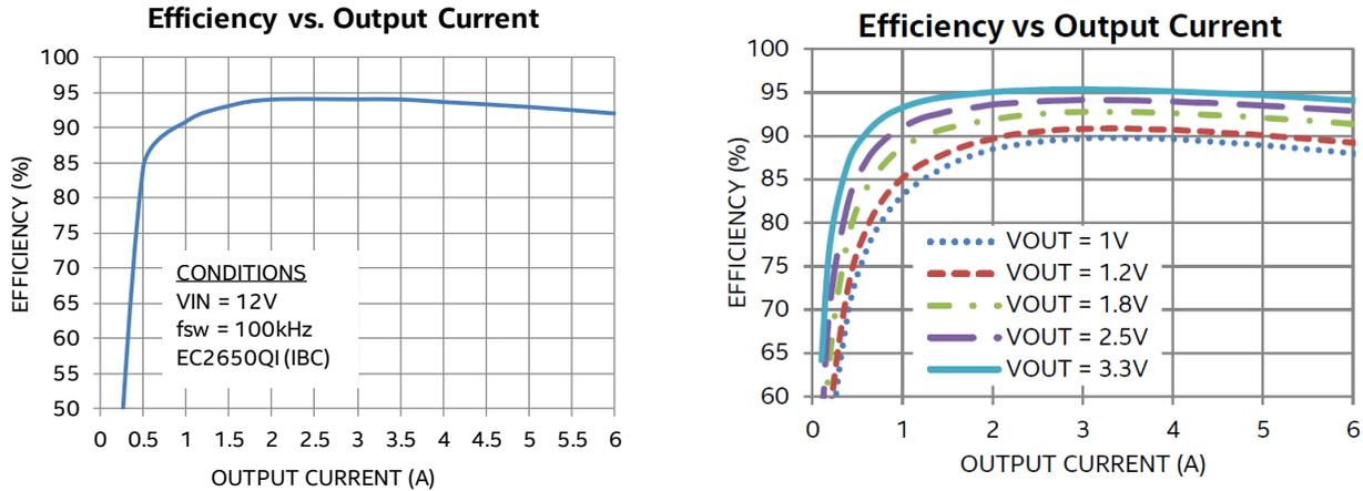
Figure 6a. EC2650QI IBC First Stage Efficiency Figure 6b. EN6362QI Second Stage Efficiency
