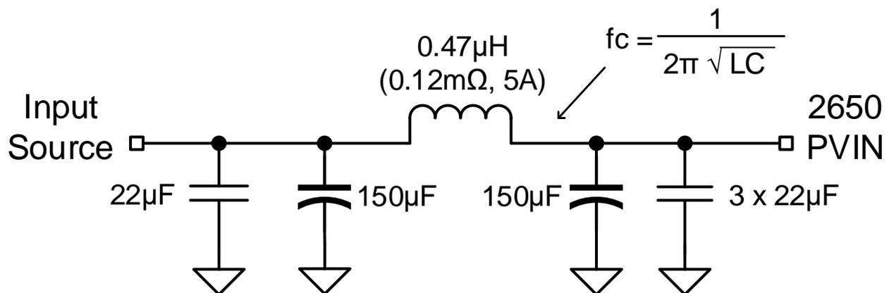
Figure 10: Input Pi Filter
