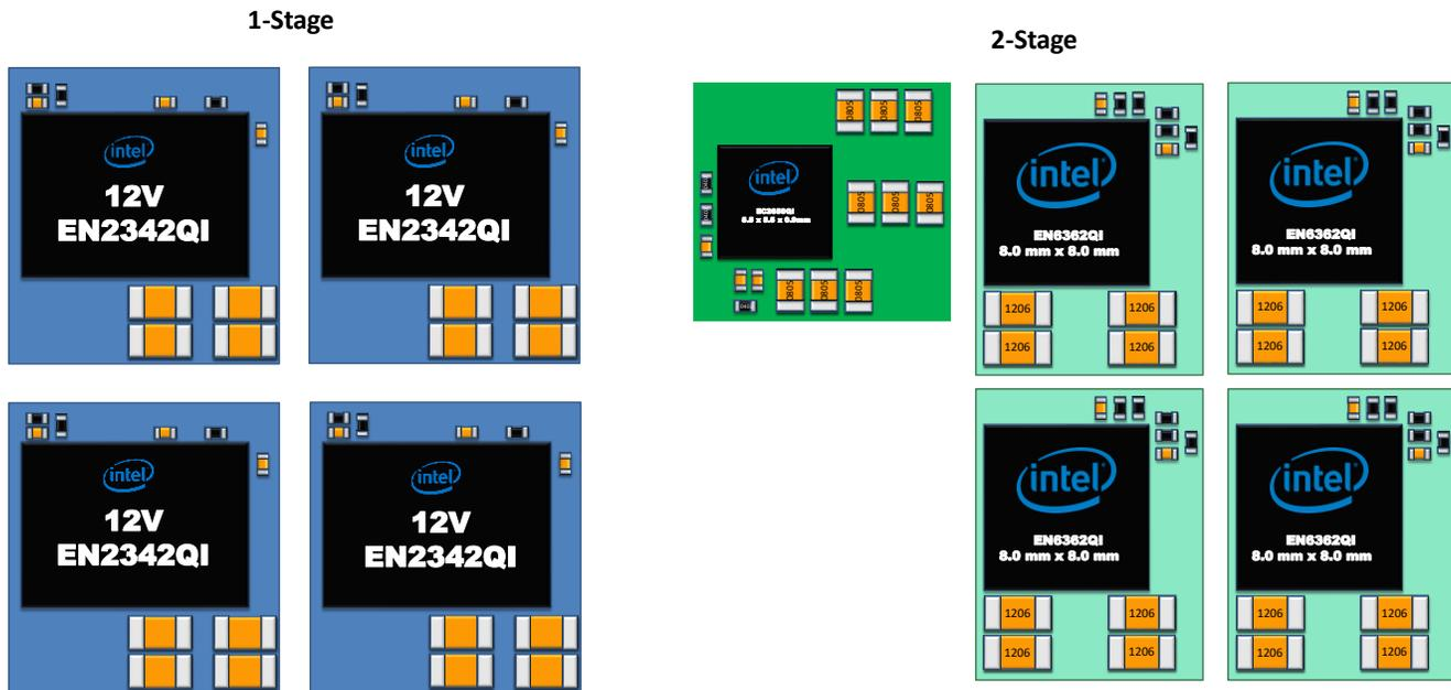
Figure 5: 1-Stage vs. 2-Stage Size Comparison with EN6362QI
