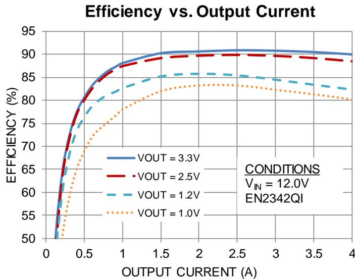
Figure 3. EN2342QI 1-Stage Efficiency
