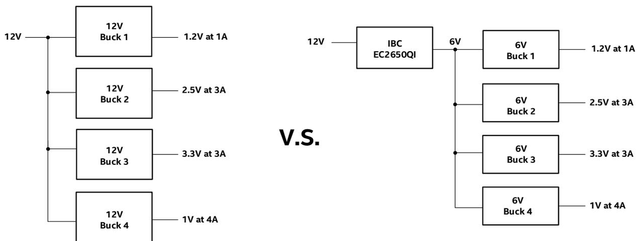
Figure 1. 1-Stage versus 2-Stage Power Tree Comparison
