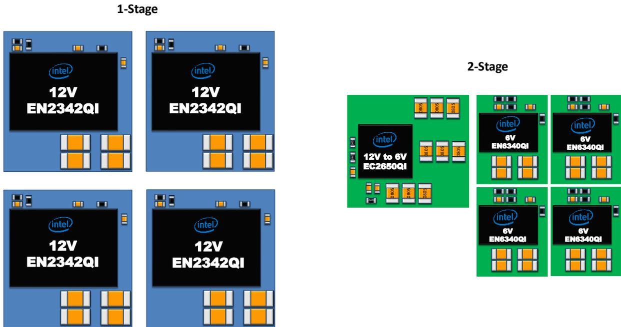
**Figure 2: 1-Stage vs. 2-Stage Layout and Solution Size Comparison**
