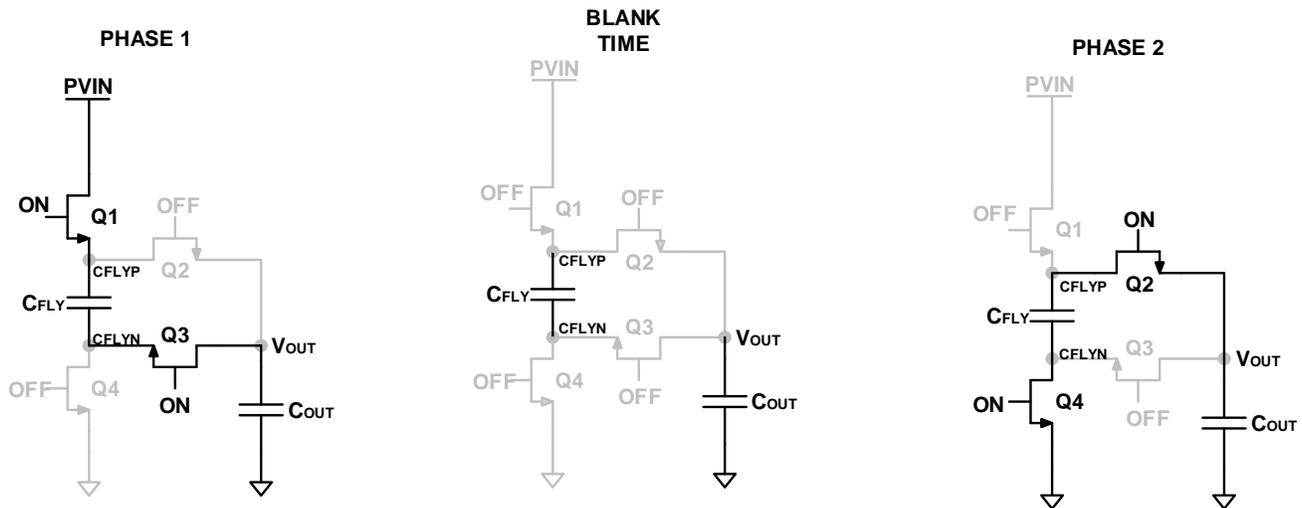
**Figure 7: Operational Switching Scheme**
