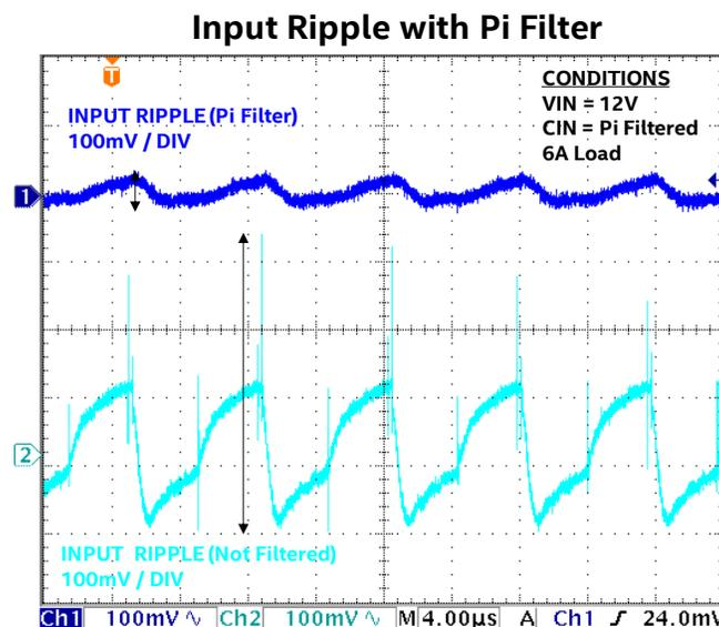
**Figure 11: Pi Filtered Input Voltage Ripple**
