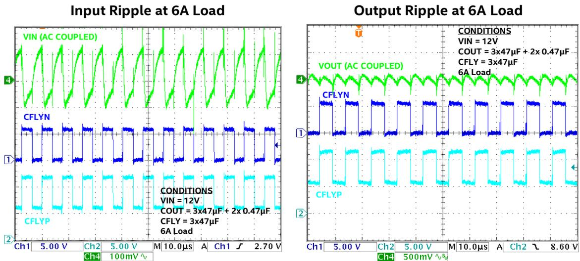
Figure 9: EC2650QI Input and Output Ripple at 6A Load
