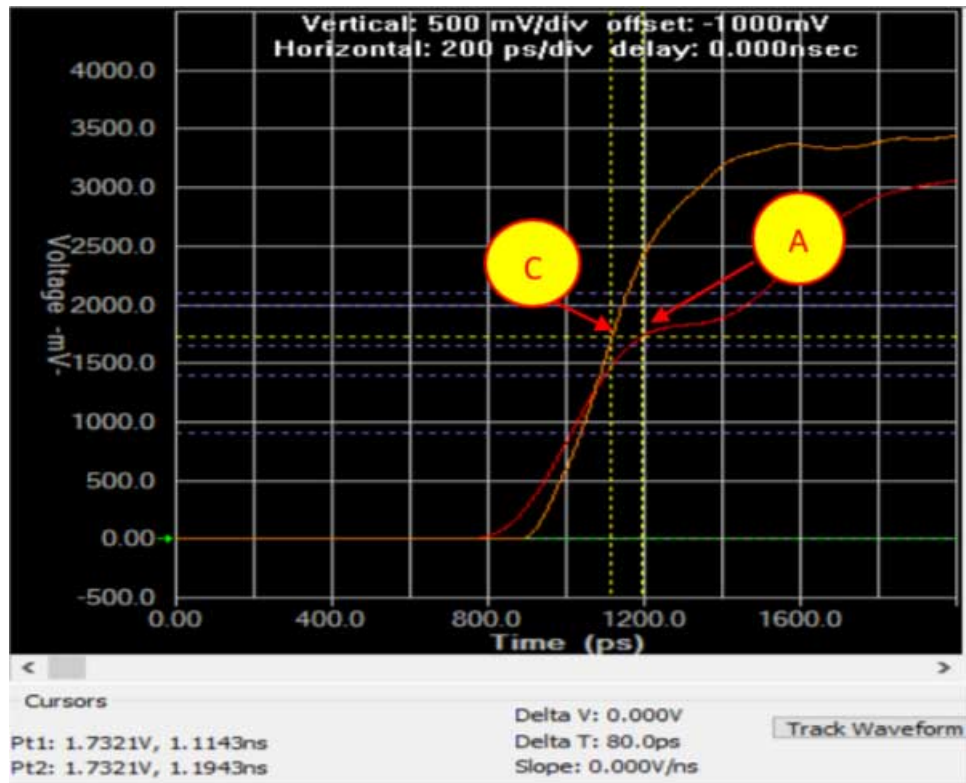
Figure 22. Minimum DCLK Delay for Delay Measurements A and C
